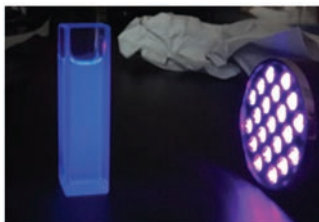
Figure 5: Carbon quantum dots made from sodium citrate.
